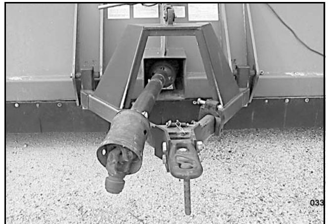
Figure 45. Pull-Type Hitch Installed
